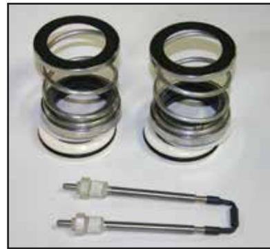
The seals are lubricated by a large capacity oil-filled chamber and protected from water leakage into the chamber with a two-conductor probe that senses and alarms water entry well before any water can enter the motor housing.
